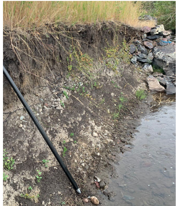
Figure 22 - Cutbanks in Subreach 3 showing stratum of fine material, maintaining a vertical bank profile, above layers with mixed gravels and fines.
